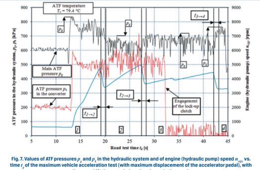
the gearshift time  $t_{i \rightarrow i+i}$  being also shown in the graph
